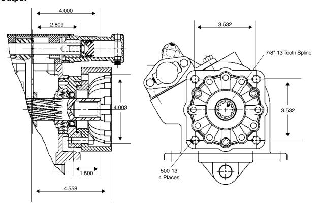
Note: "RA" and "RB" Flanges Rotate in 30º Increments
